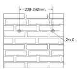
2. After cleaning the holes, place the 2 wall anchors into the holes, then attach the wall bracket to the wall using the hexagon head screw delivered with the inverter.
