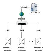
The inverter has integrated ComBox (with Ethernet module),
