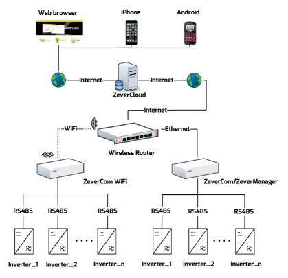
The ZeverCom/ZeverManager connects to the inverter via the RJ45 interface, and it connects to the router via Ethernet.
