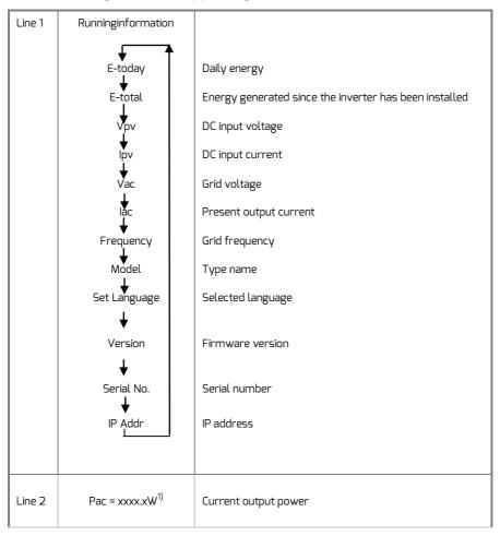
1)If the item "IP Addr" on the top line is displayed, the communication connection state with Zever Could (Disconnected or Connected) will be displayed on bottom line.
