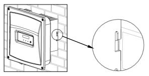
5. Pushthe inverter inwards as far as possible and attach it to both sides of the wall bracket using the M5 screws(screwdriver type: T25,torque: 2.2Nm).
